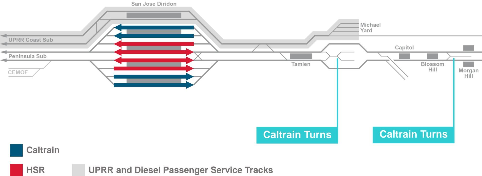
Operating all Caltrain through Diridon and turning a maximum of four trains at Tamien broadly works in currently contemplated infrastructure in PEPD and assumed changes at Diridon contemplated in DISC analysis
