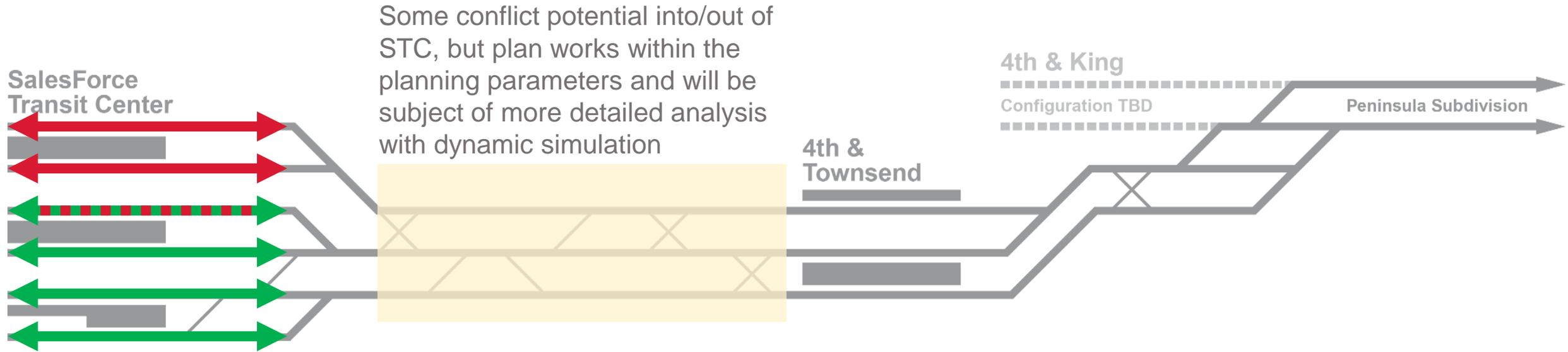
Turn times at STC above minimum requirements are achievable with HSR assigned to two tracks and Caltrain assigned to four tracks. Three and three is also achievable with tighter turns for Caltrain
