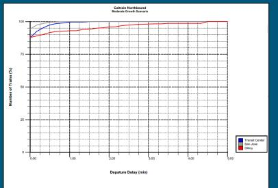
Shows, on average, northbound Caltrain trains arriving with less delay at STC than introduced at Gilroy showing ability to make up time enroute. Nearly all trains arrive with one minute of schedule to STC despite variations in dwell and added delay in the *Moderate Scenario*
