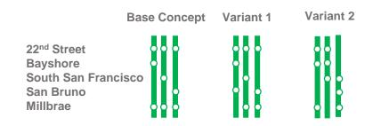
The Baseline Scenario has limited flexibility due to lack of passing tracks
