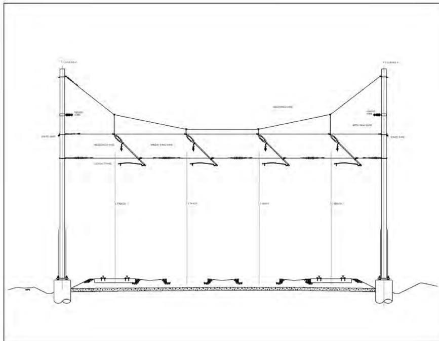
Multi-track Arrangement with Headspan Construction
