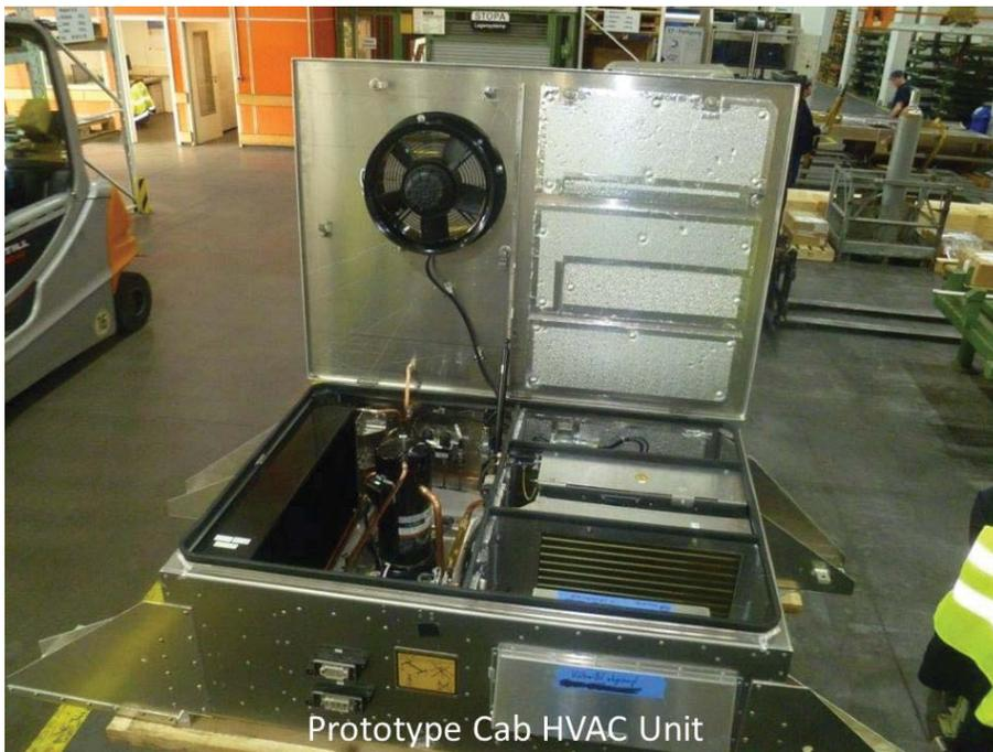
Prototype Cab HVAC Unit
