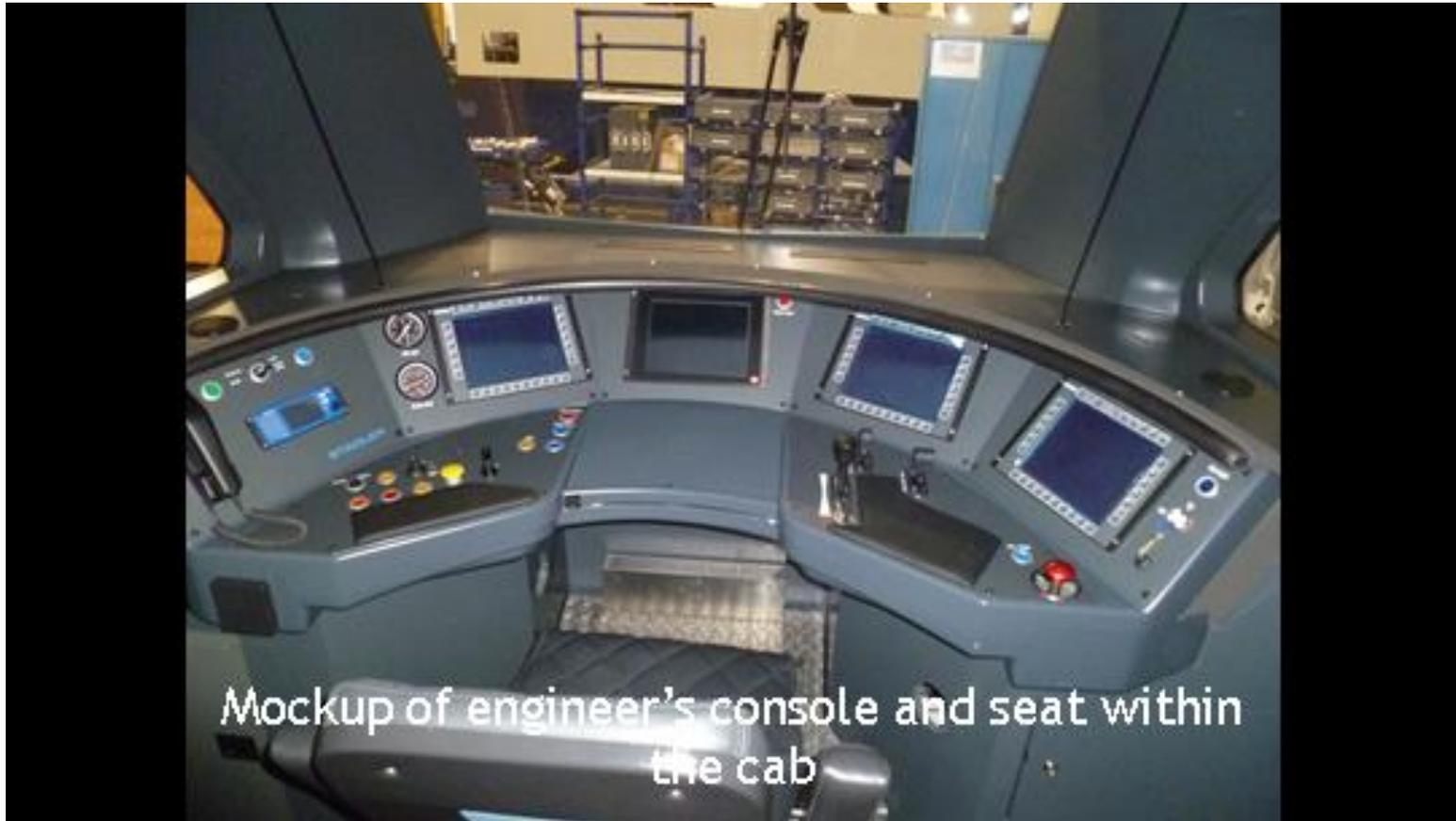
Mockup of engineer's console and seat within the cab
