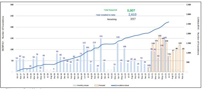
**Figure 2-5 OCS Foundation Production**
