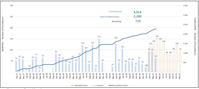
**Figure 2-5 OCS Foundation Production**
