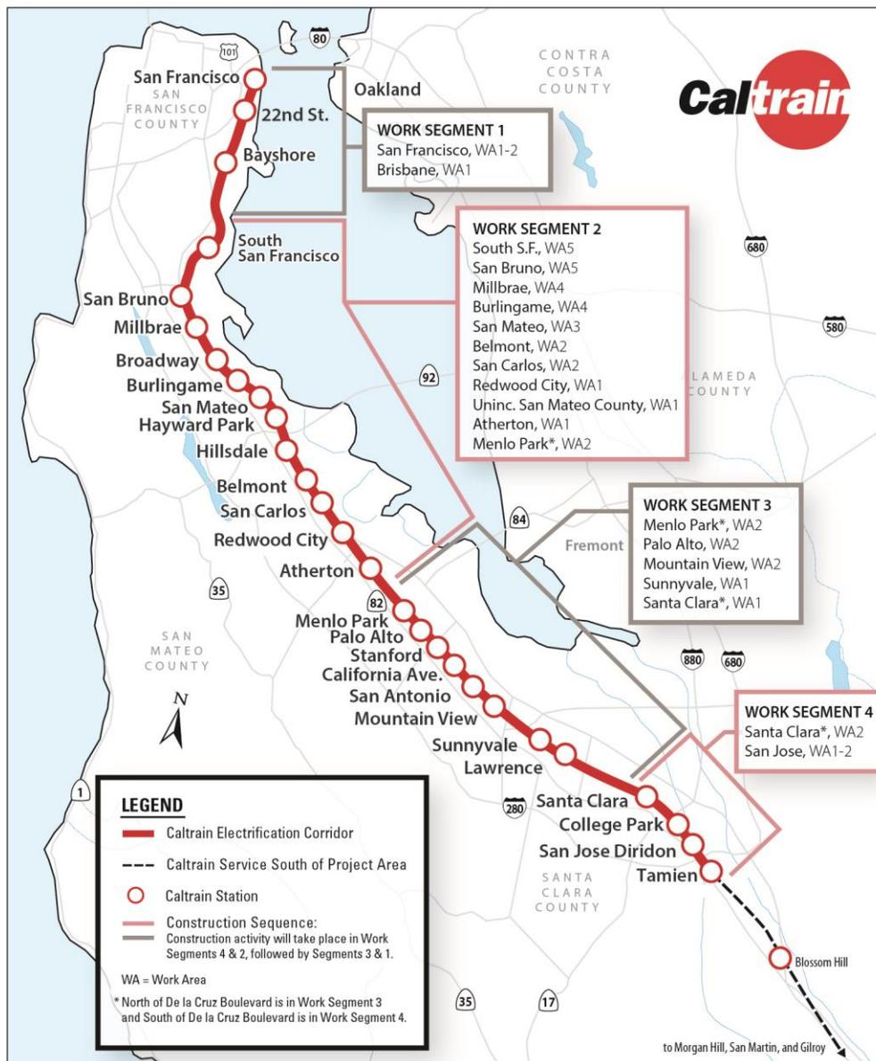
Overhead Contact System (OCS) foundation installation resumed at the end of September in Segment 2 and will continue for the next few months. Traction Power Substation (TPS) 2 construction continued with the installation of main transformers.
