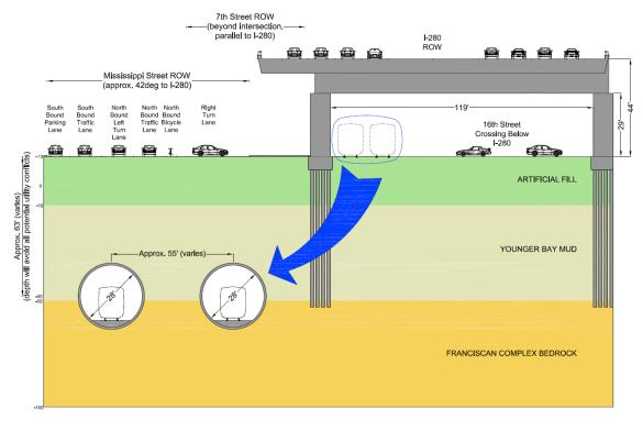
Section A-A (not to scale, example of a typical cross section, actual cross section and freeway supports vary along the alignment)
