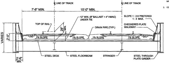
STEEL THROUGH PLATE GIRDERS NO SCALE
