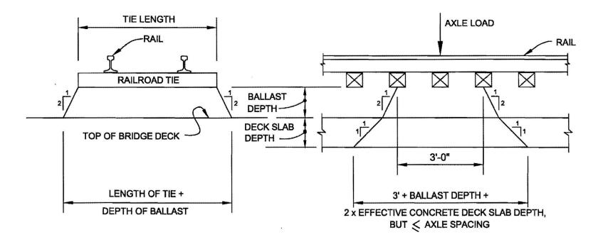
FOR CONCRETE STRUCTURAL DESIGN : LATERAL DISTRIBUTION OF LIVE LOAD TO BRIDGE DECK, PER AREMA CHAPTER 8.2.2.3.C (3)
