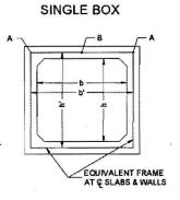
$$\begin{aligned} &Max \quad M_{B} = \frac{Wb^{2}}{24} \left(\frac{1+3k}{1+k}\right) - \frac{P_{e}h^{2}}{12} \left(\frac{k}{1+k}\right) = in \quad lb - ft, \quad use \quad min. \quad value \quad of \quad P_{e} \\ &Max \quad M_{A} = \frac{Wb^{2}}{12} \left(\frac{1}{1+k}\right) + \frac{P_{s}h^{2}}{12} \left(\frac{k}{1+k}\right) = in \quad lb - ft, \quad use \quad max. \quad value \quad of \quad P_{e} \quad or \quad P_{s} \\ &V_{A} = \frac{Wb}{2} = in \quad lbs \end{aligned}$$
