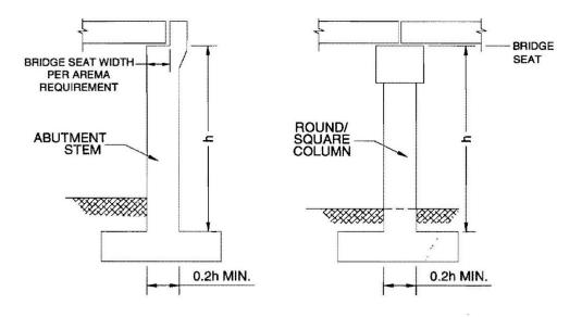
FIGURE 2.1 – ABUTMENT AND COLUMN REQUIREMENTS
