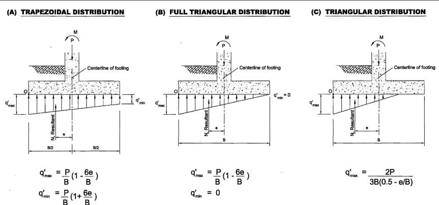
ALL PRESSURE DISTRIBUTIONS ARE BASED ON 1 FT. STRIP OF FOOTING, THESE EQUATIONS ARE RECOMMENDED FOR PRELIMINARY DESIGN.
