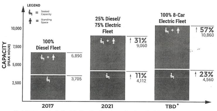
\*The CalMod program lays the foundation for continued capacity growth on the corridor. Unlike diesel trains, electric trains can maintain performance while expanding to 8-cars. Eight car expansion is dependent on additional funding.
