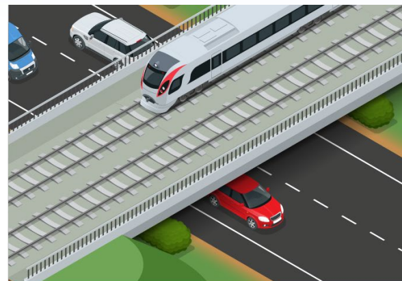
Grade Separated Crossing
