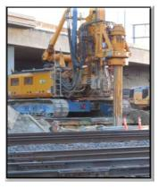
DrillTech off-track OCS Drill Rig
