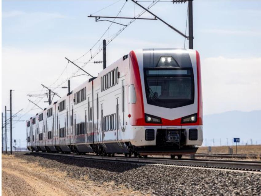
Some of the other tests completed included dynamic brake, propulsion, wheel spin and wheel slide, PTC, ride quality, abnormal service conditions, train control, network monitoring, and diagnostics. The vehicle is returning to the Salt Lake City train manufacturing facility to be prepared for travel to California. We look forward to seeing this vehicle on our property later this year.
