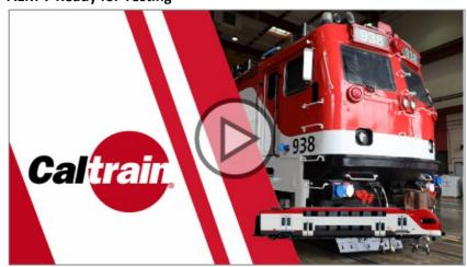
Caltrain Electrification recently added the AEM-7 (see <u>video</u>) to the project. Purchased from Amtrak, the AEM-7 will be used to test the electric catenary system which will provide power to Caltrain's electric fleet. This will ensure Caltrain that the Electrification infrastructure is in good working order before our state-of-the-art electric trains get plugged into the system, keeping the new high-performance fleet in pristine condition for electrified passenger service.
