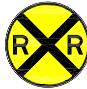
W10-1 HIGHWAY-RAIL GRADE CROSSING ADVANCE WARNING
