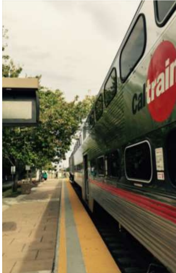
Tree encroaching within the Operating envelope
