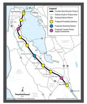
The Corridor Electrification Project is a key component of the Caltrain Modernization Program and consists of converting Caltrain from diesel-hauled to Electric Multiple Unit (EMU) trains for services between the Fourth and King Street Station in San Francisco and the Tamien Station in San Jose. The project would include the installation of new electrical infrastructure and the purchase of electrified vehicles. Caltrain will continue Gilroy service and support existing tenants.
