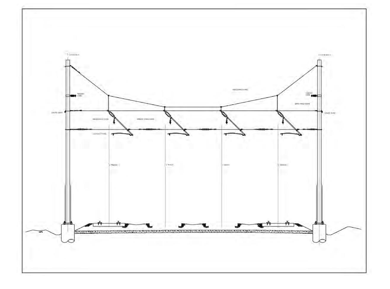
Multi-track Arrangement with Headspan Construction
