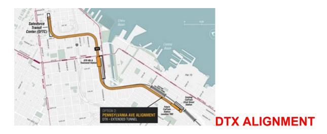
The newly-created Executive Steering Committee needs to verify that the current alignment really works for both DTX and High-Speed Rail far into the future---for constructability, length of stations relative to length of trains, fouling of tracks, operations and future expansion and technology.
